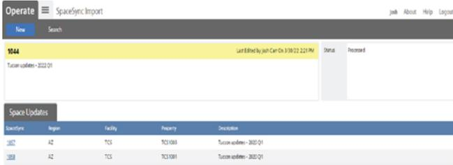
Importing can be used to create one or more SpaceSync records from an Excel file with space data in the pre-defined format.
